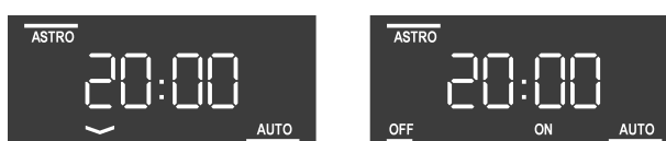
Figure 2: Automatic mode with Venetian blind or switching/dimming insert
