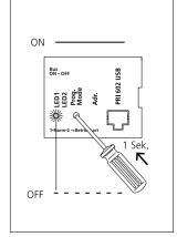
**6** Switch off the Plug+Play-mode at the BNG/BVNG 650-... by briefly pressing the programming mode key. The LED 1 at the BNG/BVNG 650-... now flashes again to indicate normal operation. All LEDs at the bus telephones are off, the system is ready for operation.
