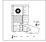
**3** Hold down the light/programming button again for 3 seconds. A short acknowledgement tone is audible. At the bus telephones, a different tone sequence is audible when a call is placed by this door station.
