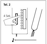
8 At the second bus telephone, hold down the internal call button you wish to use to call the first bus telephone for 4 seconds.
