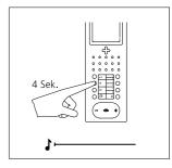
**3** Hold down the light button for 4 seconds. A prolonged acknowledgement tone is audible in the receiver, the muting button flashes. A speech connection exists to the door station. The bus telephone is now in the programming mode.
