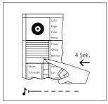
2 At the door station, hold down the light/programming button for 4 seconds. A protracted acknowledgement tone is then audible which is repeated every 5 seconds as long as the programming mode remains active.
