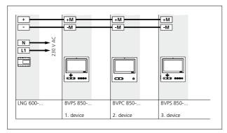
A maximum of 3 BVPS/BVPC 850-... devices can be supplied by one power line rectifier LNG 600-.... The maximum current of the 30 V DC direct voltage from the LNG 600-... is 1100 mA. The specified ranges only apply to the external power supply to the devices, not to the ranges of the In-Home bus. Ranges applicable for J-Y(ST)Y or YR installation cable with 0.8 mm core diameter! Only bus indoor devices which are located in the same line can be supplied by one line rectifier.
