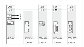
A maximum of 3 VIB 150-.../BTSV/BTCV/BFCV 850-... units can be supplied by a NG 602-... line rectifier. The maximum current of the 30 V DC direct voltage from the VNG 602-... is 1100 mA. The specified ranges only apply to the external power supply to the devices, not to the ranges of the In-Home bus. Ranges applicable for J-Y(ST)Y or YR installation cable with 0.8 mm core diameter! Only bus indoor devices which are located in the same line can be supplied by one line rectifier.
