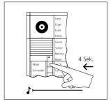
**3** At the door station, press the call button you wish to be assigned to the BSE 650-... An assignment to one or more bus telephones must exist.
