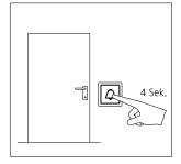
**3** Hold down the storey call button connected to the bus indoor device for 4 seconds. The bus indoor device is now in the programming mode. During this period, no ringing is admissible within the system.
