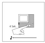
Hold down the speech button for 4 seconds. A protracted acknowledgment tone sounds as confirmation and the muting LED begins to flash. The bus indoor device establishes the speech connection to the door station. The bus indoor device is now in the programming mode.
