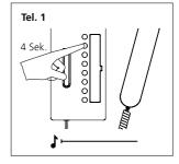
3 Lift the receiver at the bus telephone which you wish to program. Hold down the light button for 4 seconds. A protracted signal tone is audible in the receiver. A speech connection exists to the door station. The bus telephone is now in the programming mode. Do not replace the receiver!
