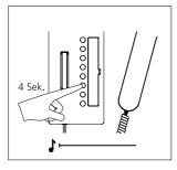
**4** Press the button you wish to program and hold down for 4 seconds. A protracted acknowledgement tone is audible in the receiver. The switching contact of the BSE 650-... is closed for 1 second.
