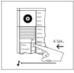
**5** At the door station, hold down the required call button for 4 seconds until a protracted tone sounds at the door loudspeaker. The call button is now assigned to the bus indoor devices, no speech connection now exists.
