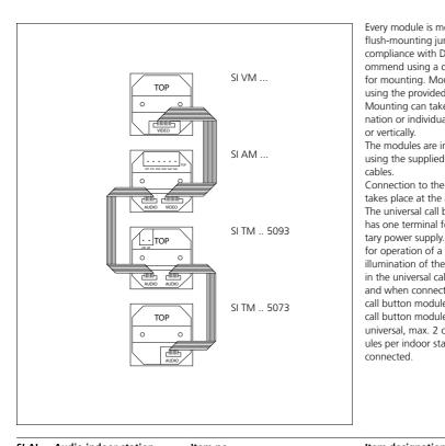
Every module is mounted in a flush-mounting junction box in compliance with DIN 49073. We recommend using a deep junction box for mounting. Mounting takes place using the provided support rings. Mounting can take place in combination or individually – horizontally or vertically.
