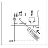
**6** Replace the receiver at all bus telephones which have been programmed. The call button is now firmly assigned to all bus telephones.
