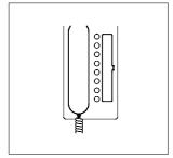
**9** Replace the receiver at both bus telephones. Program additional bus telephones using the same procedure or quit the programming mode.
