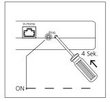
**3** Press the Prog. button on the base station for 4 seconds. The LED Prog. then flashes in a one-second rhythm. The Siedle Scope/Smart Gateway Mini is now in the programming mode.
