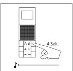
**5 Video indoor station 1:** Hold down the internal call button you wish to use to call the second device for 4 seconds.
