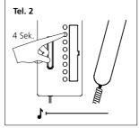
Hold the light button down for 4 seconds. The acknowledgement tone is audible. Do not replace the receiver.
