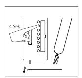
**4** Hold down the light button for 4 seconds. A protracted signal tone is audible in the receiver. The bus telephone is now in the programming mode. Do not replace the receiver! The camera picture can be seen on the monitor.
