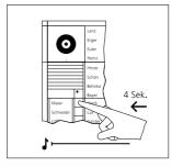
**5** At the door station, hold down the required call button for 4 seconds until a protracted tone sounds at the door loudspeaker. The call button is now assigned to the bus indoor devices, no speech connection now exists.
