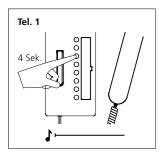
7 At the first bus telephone, hold down the internal call button you wish to use to call the second bus telephone for 4 seconds.
