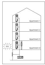
**5** Set up the bus telephone in apartment 4 with the receiver in place, the storey call sounds as an acknowledgement tone and the LED of the muting button flashes.
