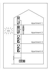
**3** Set up the bus telephone in apartment 2 with the receiver in place, the storey call sounds as an acknowledgement tone and the LED of the muting button flashes.
