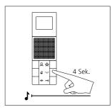
**3** Hold down the light button for 4 seconds. A protracted acknowledgement tone sounds as confirmation and the muting button begins to flash. The video indoor station establishes the speech connection to the door station. The video indoor station is now in the programming mode.
