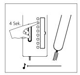
4 Hold down the light button for 4 seconds. A protracted acknowledgement tone sounds in the receiver, the muting button flashes. A speech connection exists to the door station. The bus telephone is now in the programming mode. Leave the receiver off the hook.
