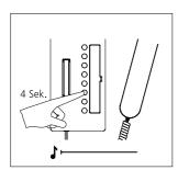
**4** Lift the receiver at the bus telephone at which you wish to program a button. Press the button you wish to program and hold down for 4 seconds.
