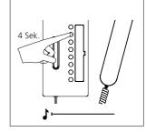
3 Lift the receiver at the bus telephone which you wish to program. Hold down the light button for 4 seconds. A protracted acknowledgement tone sounds in the receiver, the muting button flashes. A speech connection exists to the door station. The bus telephone is now in the programming mode. Leave the receiver off the hook.
