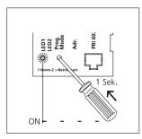
Switch on the programming mode. At the BNG/BVNG 650-..., press the programming mode button briefly. The LED 1 flashes in a 2-second rhythm to indicate that the programming mode is active.
