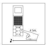
**3 Video indoor station 2:** Hold down the light button for 4 seconds. A protracted acknowledgement tone sounds as confirmation and the muting button begins to flash.
