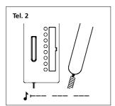
Lift the receiver at the second bus telephone you wish to enable for internal calls. The programming mode tone is audible.
