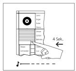
At the door station, hold down the light/programming button for 4 seconds. A protracted acknowledgement tone is then audible which is repeated every 5 seconds as long as the programming mode remains active.
