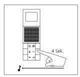
**2 Video indoor station 1:**Hold down the light button for 4 seconds. A protracted acknowledgement tone sounds as confirmation and the muting button begins to flash.
