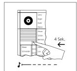
**2** At the door station, hold down the light/programming button for 4 seconds. A protracted acknowledgement tone is then audible which is repeated every 5 seconds as long as the programming mode remains active.
