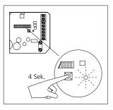
2 At the BVA 650-... hold the programming button down for 4 seconds. After this, the status LED flashes at short intervals as long as the programming mode is active.
