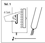
Hold the light button down for 4 seconds. The acknowledgement tone is audible. Do not replace the receiver.
