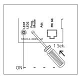
**1** Switch on the programming mode. At the BNG/BVNG 650-..., press the programming mode button briefly. The LED 1 flashes in a 2-second rhythm to indicate that the programming mode is active.
