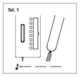
Lift the receiver at the first bus telephone you wish to enable for internal calls. The programming mode tone is audible.
