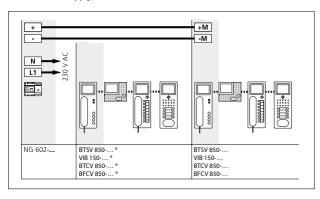
A maximum of 1 VIB 150-.../BTSV/BTCV/BFCV 850-... unit can be supplied by a NG 602-... line rectifier. The maximum current of the 24 V DC direct voltage at the NG 602-... is 300 mA. If several bus telephones have to be simultaneously rung using one bell button, each VIB 150-.../BTSV/BTCV/BFCV 850-... must have its own NG 602-... Alternatively, up to 3 bus telephones with colour monitor can be supplied from a video line rectifier VNG 602-...
