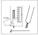
**5** At the bus telephone, hold down the button you wish to use to call the door station for 4 seconds. Replace the receiver. The button is now assigned to the door station. The door loudspeaker can be dialled at any time.
