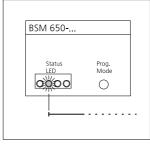
**3** Select the relevant relay by actuating the Prog. mode button at the BSM 650-... with a screwdriver until the required LED lights up (LED2 = relay2, press 2x).
