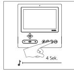
**3** Hold down the light button for 4 seconds. A protracted acknowledgment tone sounds as confirmation and the muting button begins to flash. The standard bus video panel establishes the speech connection to the door station. The standard bus video panel is now in the programming mode.
