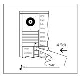
At the door station, hold down the required call button for 4 seconds until a protracted tone sounds at the door loudspeaker. The call button is now assigned to the bus indoor devices, no speech connection now exists.
